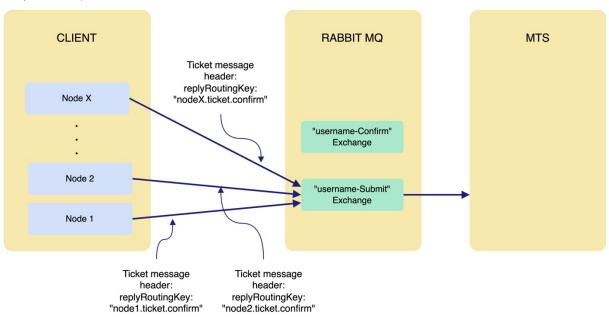
However, the ticket response must be sent exactly to the node from which the ticket originated. This is achieved by multiple Confirm queues (each of them designated for a particular node) and the replyRoutingKey. Every ticket that is submitted to the Submit exchange must contain the replyRoutingKey in the message header. This key will be used by MTS as the Routing Key when submitting the response to the Confirm exchange.
